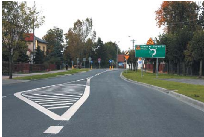
Photograph 9. At the three-entrance junction with the road to Przewóz Stary, a roundabout was also constructed, which might give rise to some controversy (such a solution was applied at the junction with DW 736).
